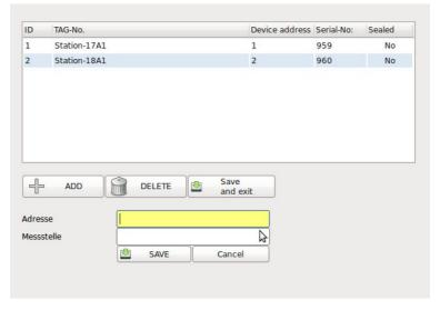
Click on Add and at first enter the Modbus address and the measuring point name of the connected Batching Master.
