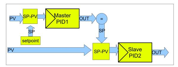
The manipulated out from master controller is the setpoint from slave controller. The first parameter set (KP1, Kd1, Tn1, Yo1, Tv1) applies to the master controller, the second parameter set (KP2, Kd2, Tn2, Yo2, Tv2) to the slave controller.
