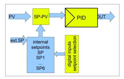
See structure menu: 6.7 Input selection for remote setpoint see input and output menu: 10.2.1
