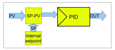
A setpoint adjustment with the arrow keys is only possible in automatic mode. In manual mode, the manipulated output will be adjusted.
