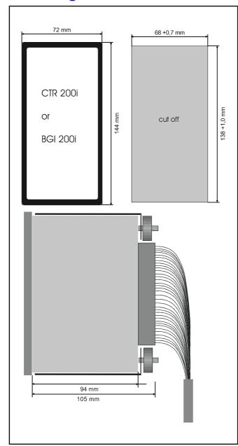
The CTR 210 has external dimensions of 144 mm x 72 mm.
