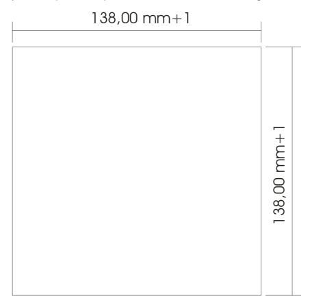
Release the two mounting profile screws. Shift the mounting profiles backwards from the panel mounting housing. Move the *Batching Master 210i* from the front side through the cut off in the panel mount. If the IP65 front is ordered, put the gasket to the Batching Master before setting in the cut off.
