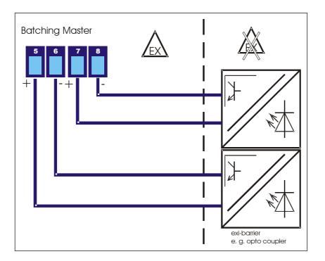
The pulse input supplies a constant current of approx. 3 mA. The maximum voltage that can be measured is approximately 5.6 V. Please note that terminals 6 and 8 must not be connected to ground and not to the same potential.
