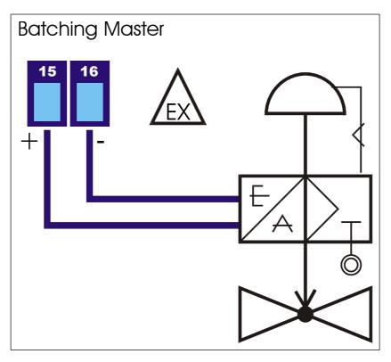
The current output is switched off when the emergency stop switch is operated.
